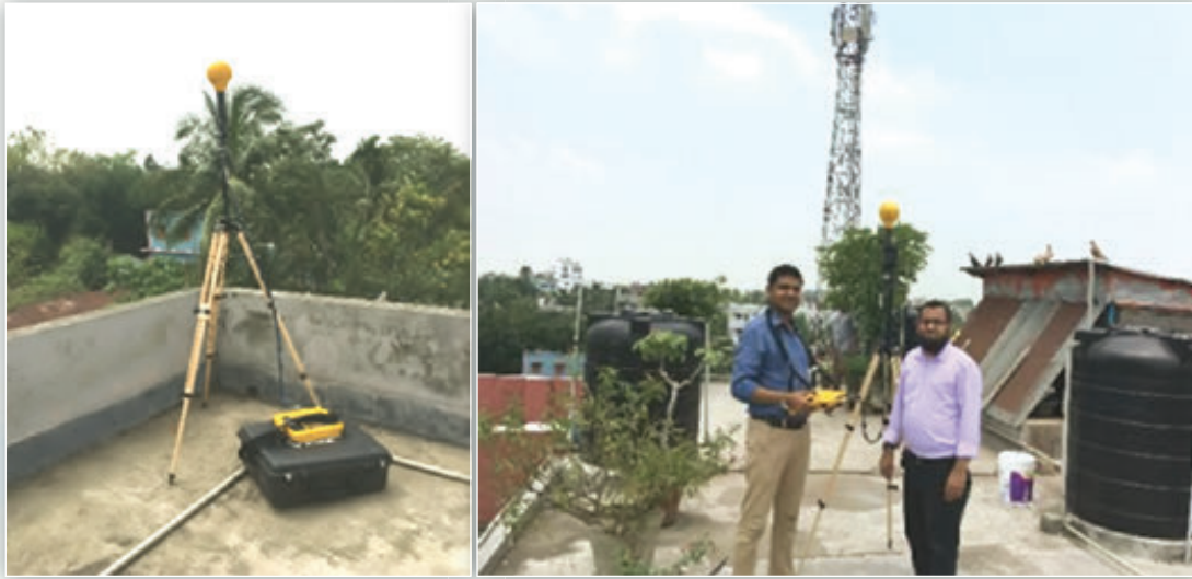
Officials of E&O, BTRC are conducting EMF-Radiation Measurement activities at various locations.
